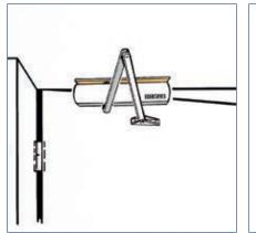
TS 4000 Transom installation/opposite hinge side lintel casing bracket
