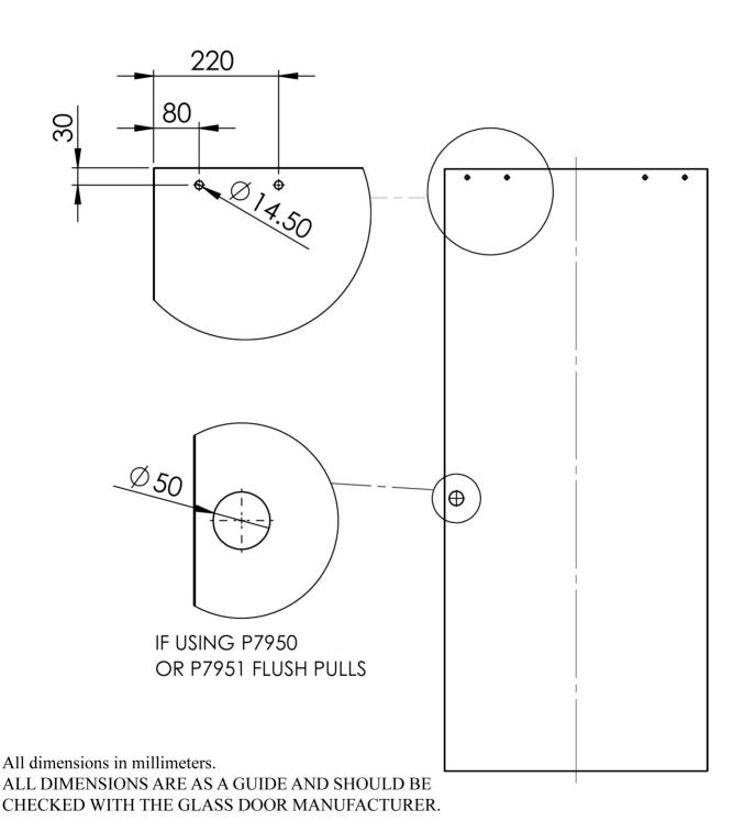
NOTE; A NARROW STRESS RELIEF SLOT MAY BE REQUIRED FROM THE RIM OF THE HOLES TO THE TOP EDGE WITH SOME GLASS TYPES. CHECK WITH GLASS DOOR MANUFACTURER.
