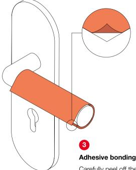
Carefully peel off the backing paper by pulling it flat back on itself and stick the tape on so that the beginning and end of the tape meet at the bottom of the handle. Slide the tape from the middle outwards into final position.
